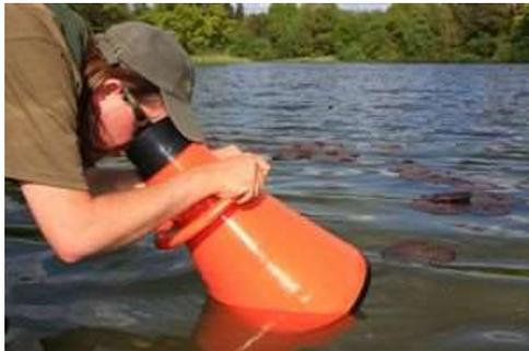
These are great for observing aquatic plant and animal life under the water. The larger aquascopes (as above) are perfect for use over the side of a small launch whilst the smaller ones would be ideal for use from the side of craft such as a canoe.
